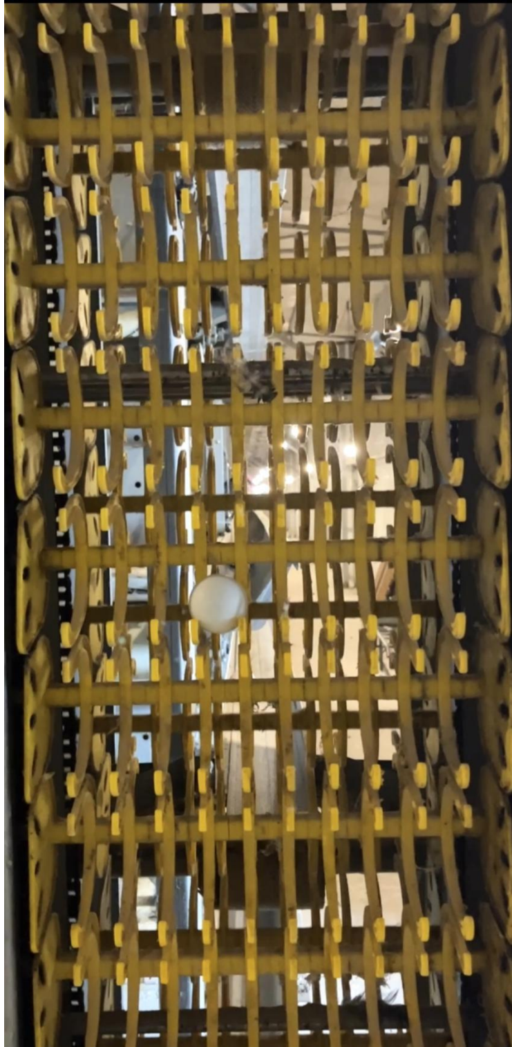
Automatic delivery chain of eggs
