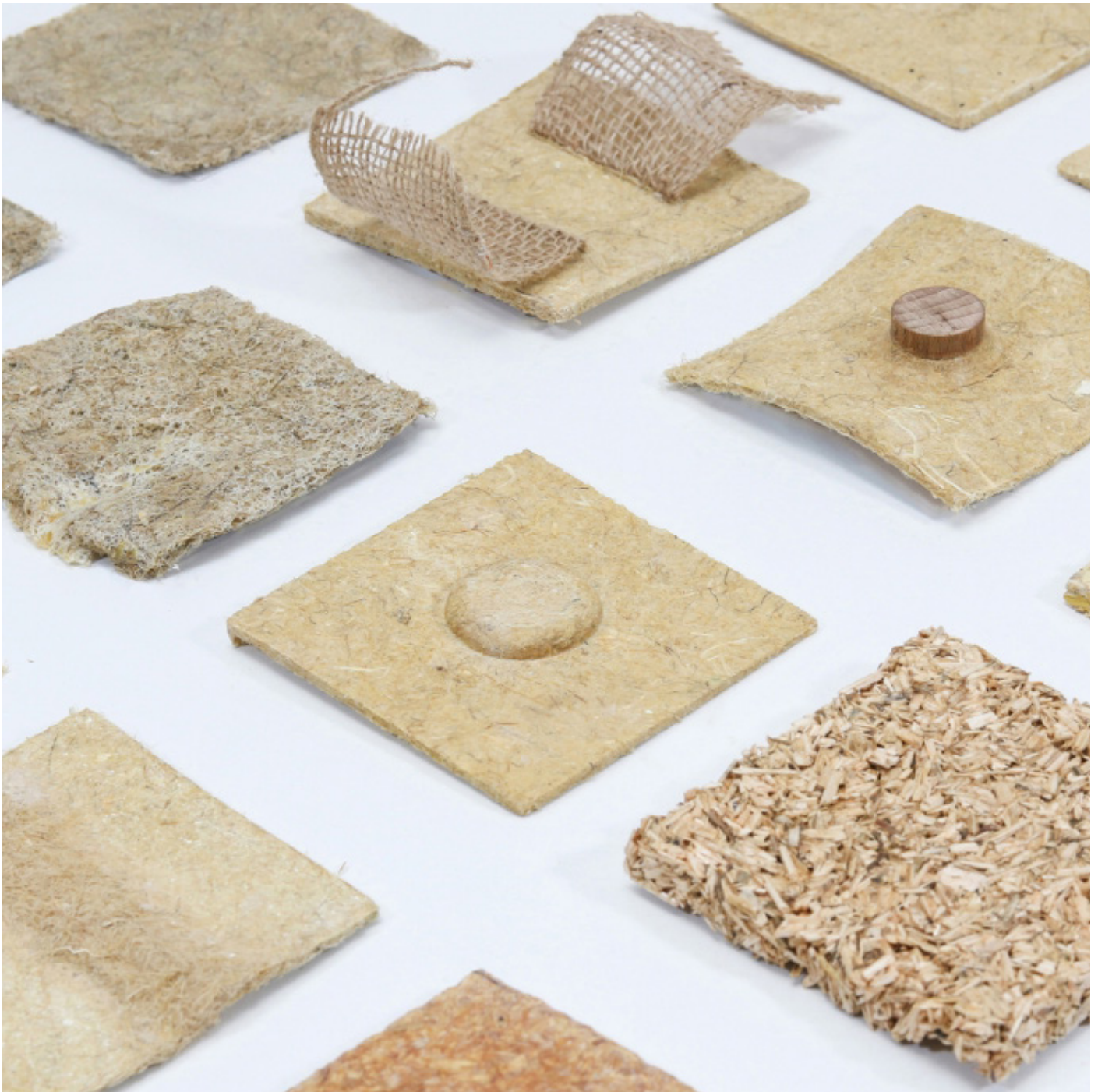
Figure 6: Organico by Philipp Hainke. Philipp Hainke is a product designer that combines an artistic background with technical solutions. His project Organico utilises traditional and renewable resources for the development of a new, innovative material. An adhesive, composed of calcium hydroxide and casein is used to press hemp fibres and shives into solid forms.
